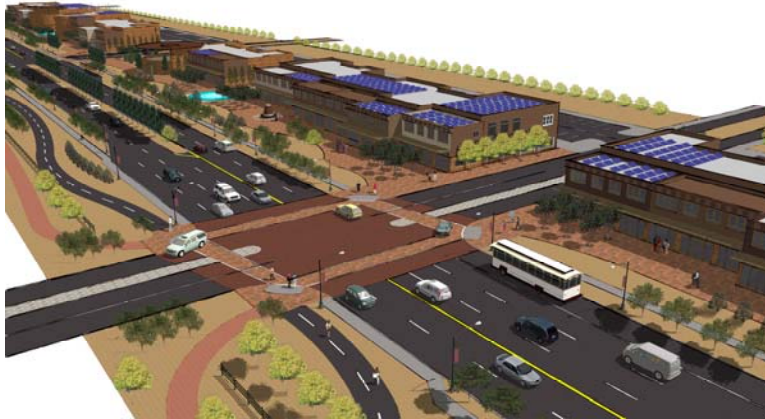
Safe At-Grade Pedestrian, Bicycle, and Equestrian Crossing Concept Connecting the Kayenta Civic Center and the Kayenta Main Street
