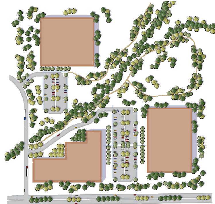
Concept Showing a Business Park with a Shared Entry Drive that Offers Limited Access
