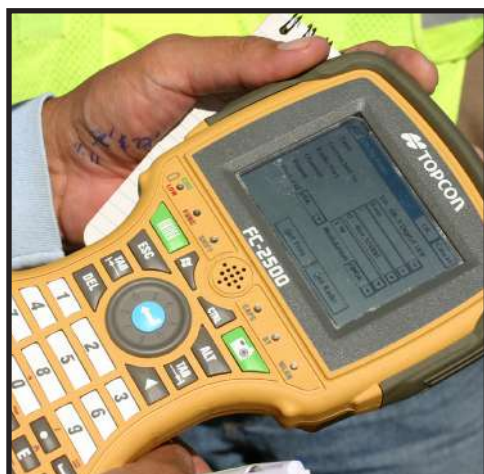
All data collected from GPS satellites from the field survey are stored in the data collector.
